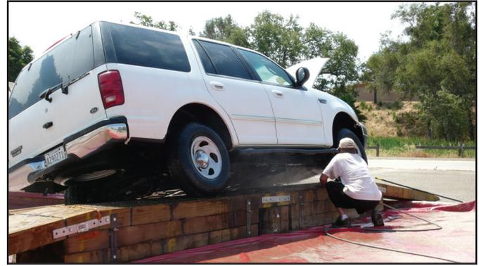
Figure 6—Cleaning ramp photo.
